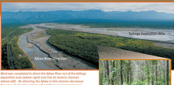
the amount of water entering the tailings management area. The tailings in the foreground of the picture were deposited before the diversion and are being reclaimed.
